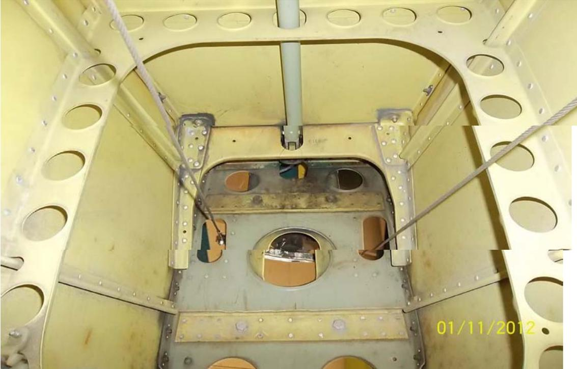
**Cessna 208B, Cracked Bulkhead, ATA 5312**
